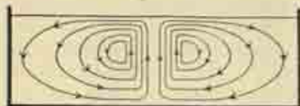
FIG. 6 Convection currents in a layer of liquid uniformly heated from below
